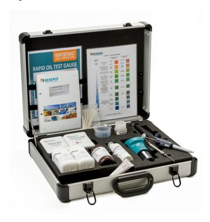
The GESERCO TAN + BN Test Kit is a true portable lubricant analysis mini laboratory.
